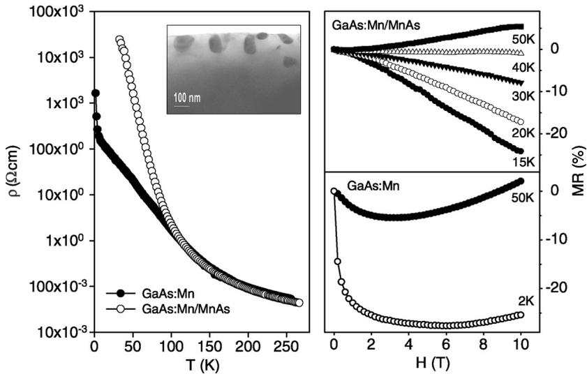
Fig. 1. Left: Temperature dependence of the resistance of paramagnetic GaAs:Mn and GaAs:Mn/MnAs hybrids. Inset: TEM image of the MnAs clusters in a GaAs:Mn matrix. Right: MR curves at various temperatures for GaAs:Mn/MnAs hybrids (top) and GaAs:Mn (bottom).
