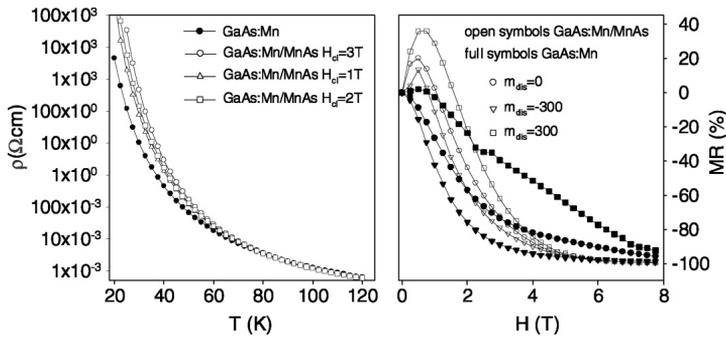
Fig. 3. Left: Calculated temperature dependence of the resistivity of paramagnetic GaAs:Mn and GaAs:Mn/MnAs hybrids. Right: Calculated MR curves for paramagnetic GaAs:Mn and GaAs:Mn/MnAs hybrids for various field-independent disorder parameters at  $T = 30$  K.
