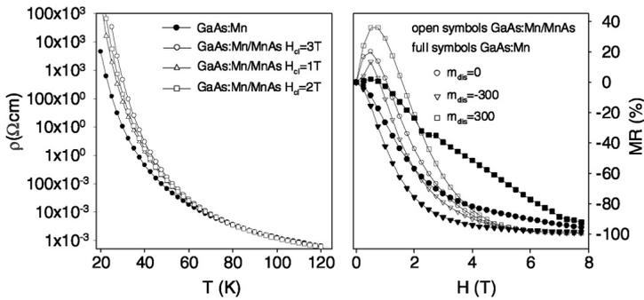
Fig. 3. Left: Calculated temperature dependence of the resistivity of paramagnetic GaAs:Mn and GaAs:Mn/MnAs hybrids. Right: Calculated MR curves for paramagnetic GaAs:Mn and GaAs:Mn/MnAs hybrids for various field-independent disorder parameters at  $T = 30\text{ K}$ .
