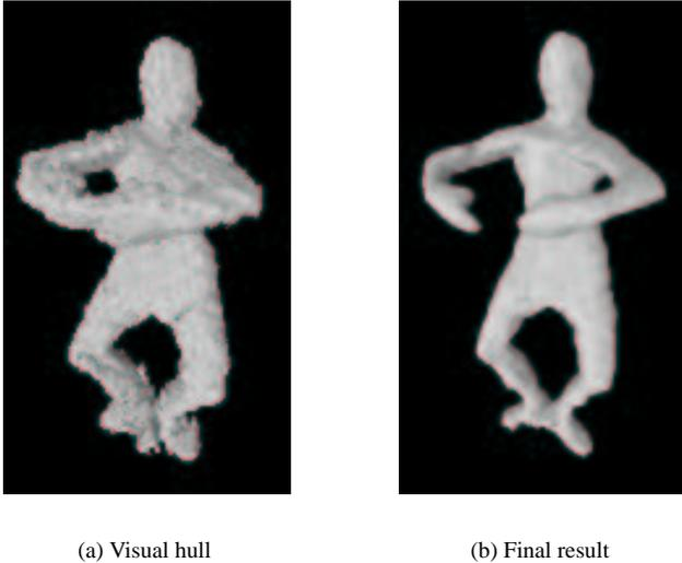
**Figure 5.** *Reconstruction: The object’s visual hull is used as the initial surface to start the PDE evolution. On the right, the final result is depicted after running the complete algorithm including normal optimization.*
