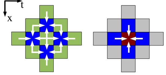
**Figure 2.** Evaluation of the differential operator. In the first step, the values of  $u_i$  in the light cells are used to compute the level set normal  $\mathbf{n} \in \mathbb{R}^4$  in the dark cells using central differences. For the second step, we compute the values for the central cell, also using finite differences.
