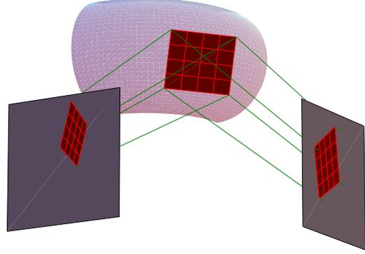
**Figure 1.** Practical computation of the cross-correlation error term  $\Phi^G$ : A small region in the tangent plane is projected into both camera images, and the normalized cross-correlation is computed.
