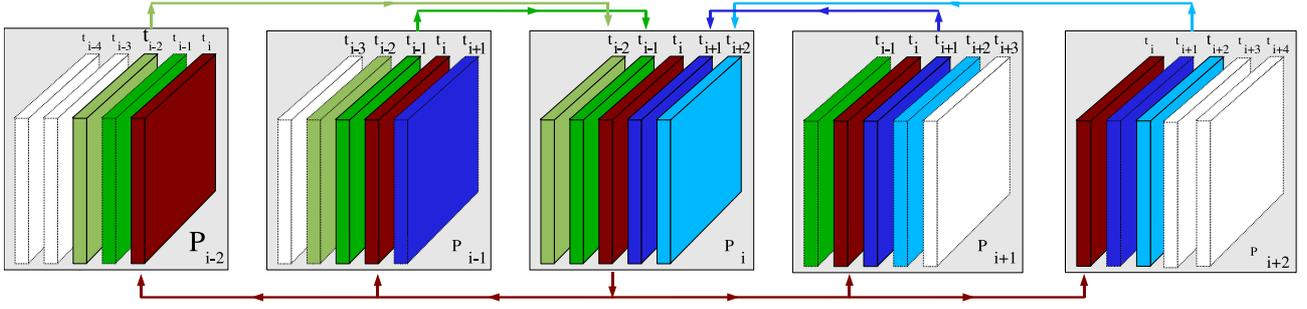
**Figure 3.** Data transmission of process  $P_i$  before an iteration. Each process stores five slices of constant time and is responsible for the computation of the center slice.  $P_i$  computed its slice in the last iteration and now transmits it over the network. On the other hand, it receives the other slices from its neighbors for the next iteration. In the figure, slices of the same color contain the same information after the communication.
