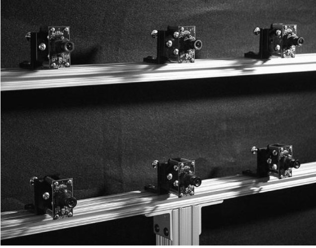
Figure 1: The Stanford Light Field Video Camera consists of numerous CMOS camera heads, arranged in a planar matrix and with aligned optical axes.
