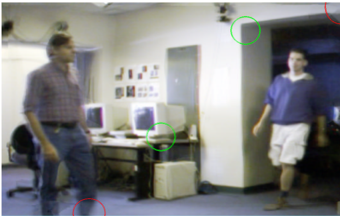
Figure 9: The predicted view from a viewpoint in the center between the four cameras. Note the sharp reproduction of features circled green. The visible blurriness in areas marked red is caused partly by motion blur in the source images and partly by inaccuracies in the depth maps as explained in the main text.
