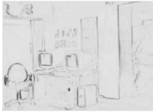
Figure 7: Residual error of disparity compensation: The error is concentrated in edges of the image, where large differences in color stem from only small inaccuracies in disparity.
