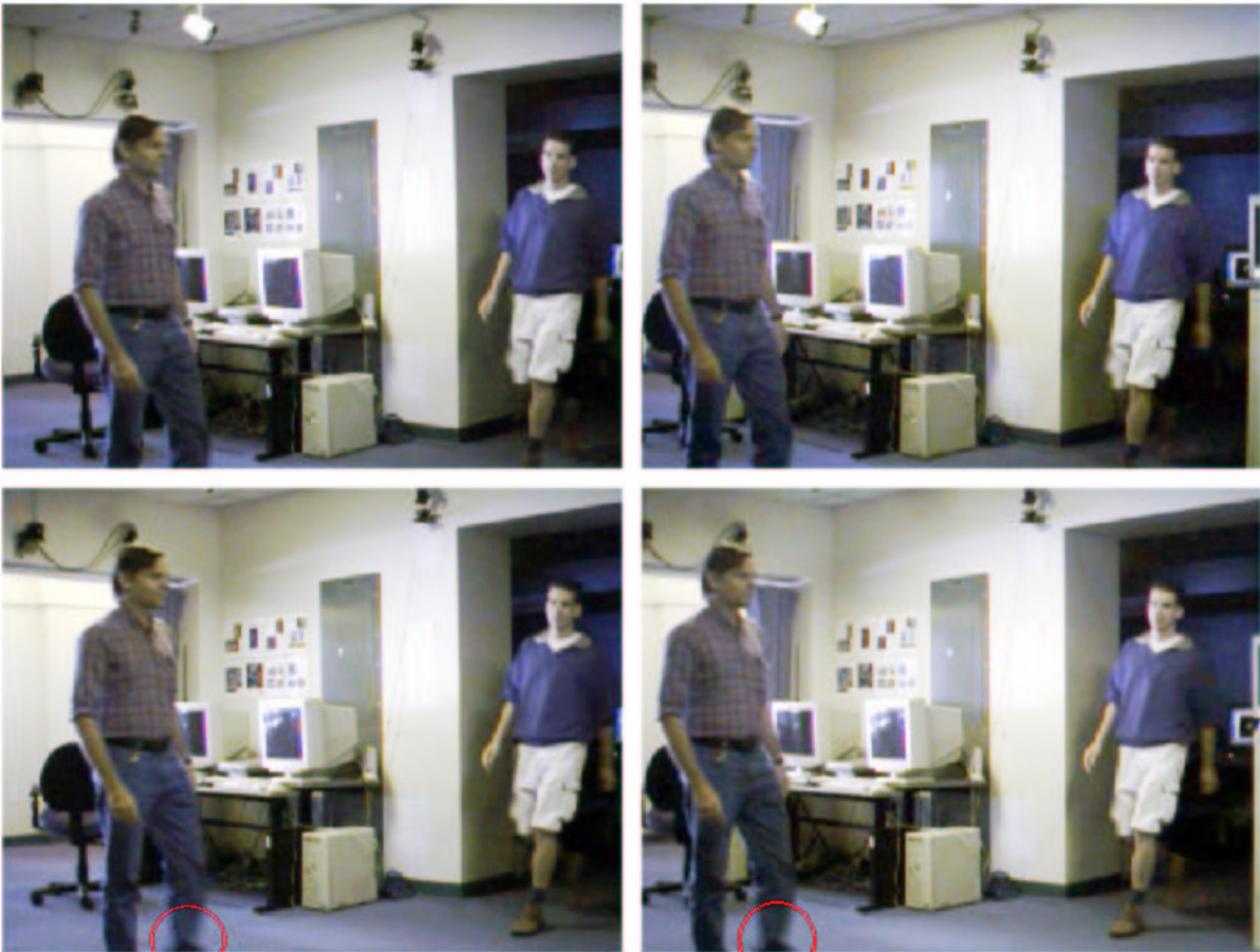
Figure 8: Source images taken by four cameras positioned at the vertices of a square. Note the artifacts circled red caused by motion blur, which lead to blurred reproduction in the predicted view below.
