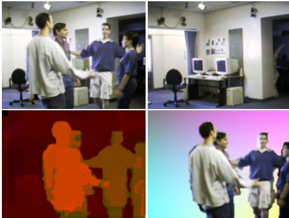
Figure 3: Top : Scene image and background image captured by a CMOS camera. Bottom : The reconstructed depth labels and the detected foreground.
