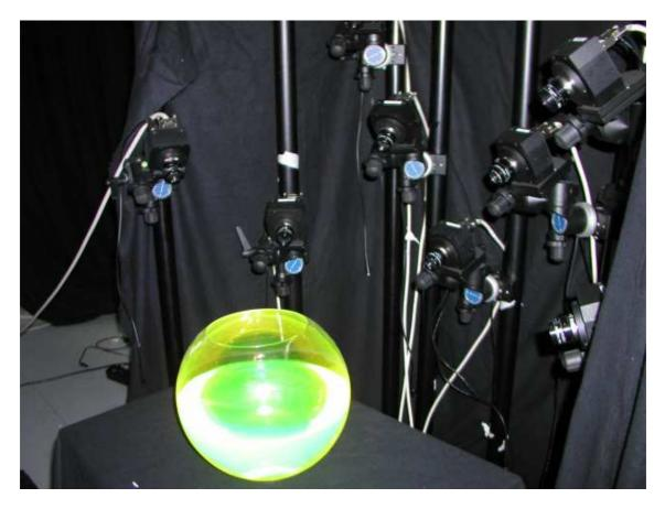
**Fig. 10.8.** Our studio setup consists of eight cameras, a fish bowl filled with dyed water and a UV light source (not visible).
